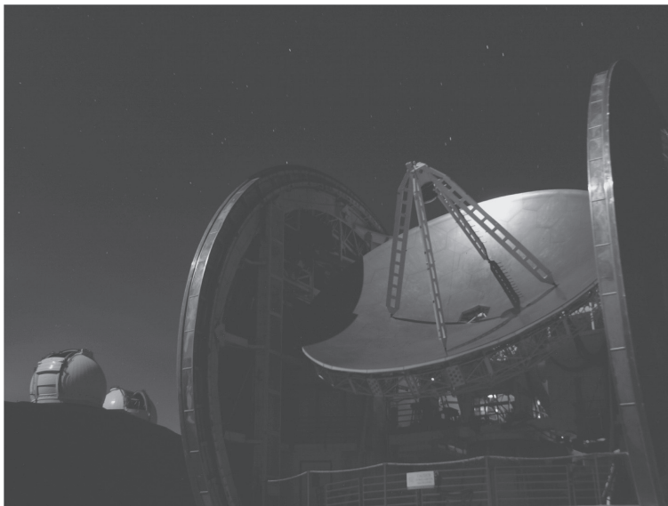
Figure 1. The Caltech Submillimeter Observatory (CSO) on top of Mauna Kea, Hawaii under full moon light. The 10.4 m diameter radio telescope was designed and assembled by a team led by Caltech Prof. Robert Leighton. In the background are the two Keck optical telescopes (10 m diameter, with hexagonal segment primary mirrors).
